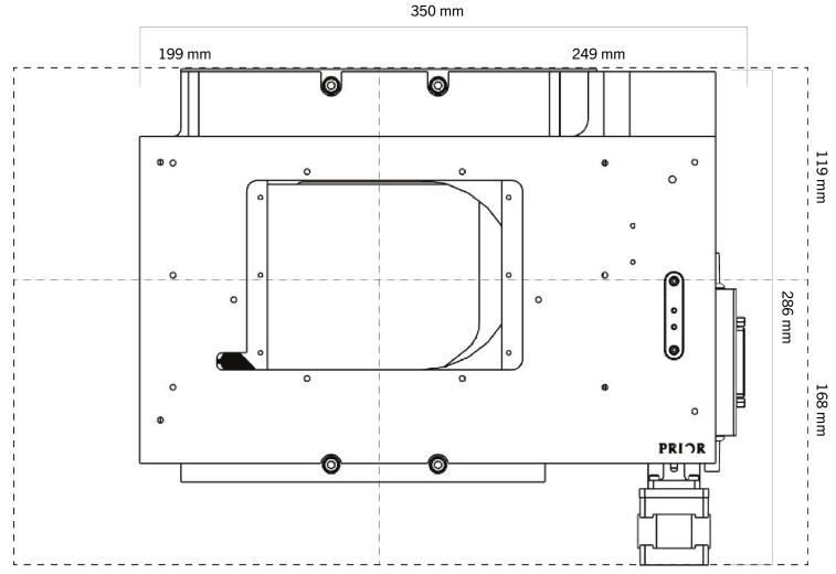
\*Outer dotted line shows the maximum footprint of the stage when at the limits of travel.
